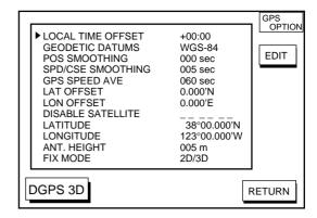
Figure 10-7 GPS SETUP options menu
